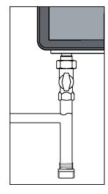
The gas supply connection must comply with local regulations or, if such regulations do not exist, with the National Fuel Gas Code, ANSI Z 223.1.
