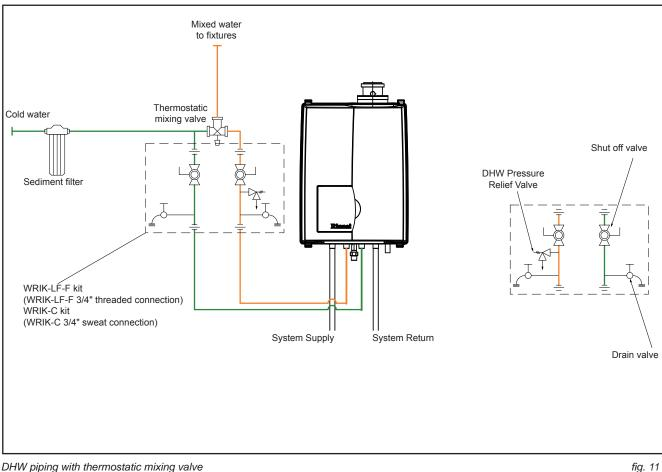
DHW piping with thermostatic mixing valve
