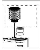
placing air filter on air intake figure 18
