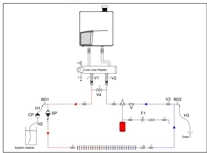
Boiler system flushing figure 9
