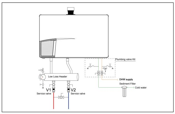
Boiler DHW piping figure 13
