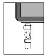
Gas shut off valve onto boiler figure 11
